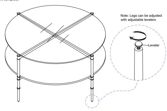
ADDITIONAL NOTE ABOUT SAFETY: BOLTS MAY LOOSEN DURING NORMAL EVERYDAY USE. THEY SHOULD BE PERIODICALLY INSPECTED AND RE-TIGHTENED TO PREVENT DAMAGE OR INJURY. ALWAYS CHECK TO ENSURE THAT ALL HARDWARE IS KEPT TIGHTENED.
