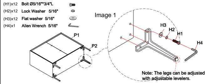
Step 2. Securely tighten all bolts with Allen wrench (H4). Turn the assembled chest to an upright position. Attach the handles (P3) to the door front as shown below image 2, **do not over tighten the screw**. Assembly is complete. **Failure to follow these instructions may cause the bolts to misalign during assembly.**
