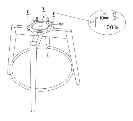
Step 4. Lay chair on side and then attach the swivel (P5) to the bottom chair seat(P1) with bolts(H1), flat washers(H3) and tighten all bolts securely with allen wrench(H4) as illustration below.
