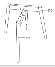
Step 2. Insert ring(P4) to leg frame(P2&P3) using bolts(H2) and fully tighten bolts with allen wrench(H4). as illustration below.
