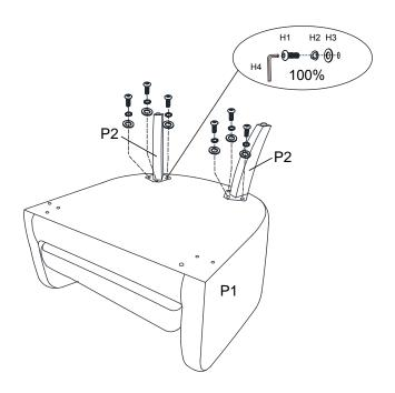
Step 2. Put on the front legs(P3), fully tighten bolts (H1) & washers(H2&H3) with allen wrench (H4) as illustration below.
