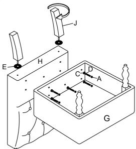
Step 4: Fully tighten all bolts . Assembly is complete.
