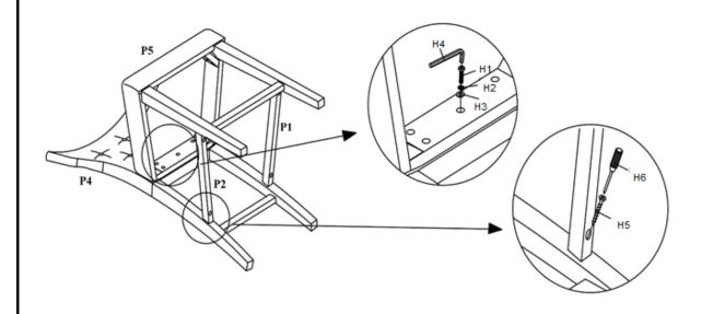
Step 5 : Fully tighten all the bolts and screws with Allen Wrench (H4) anad Screwdriver (H6) before turning the chair over and place it upright on a level surface. Assembly is completed .
