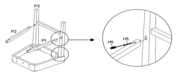
Step 3 : Attach Step - 2 assembled part to the Back Leg Frame (P4) as shown below :
