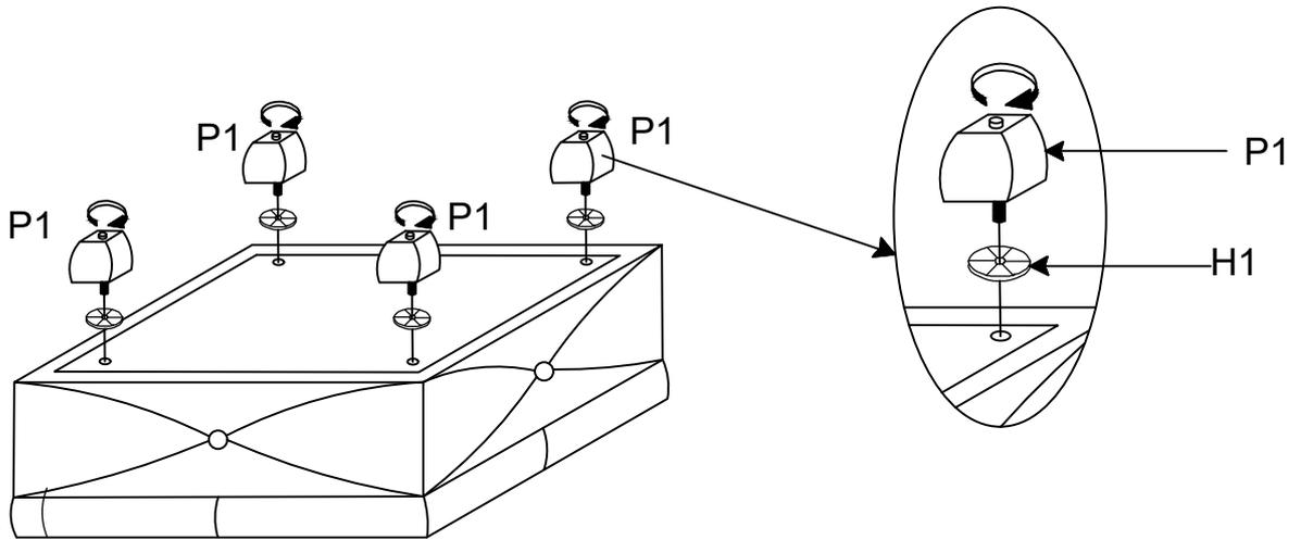
Step 3. Level the storage box and place it upright on a level surface.
