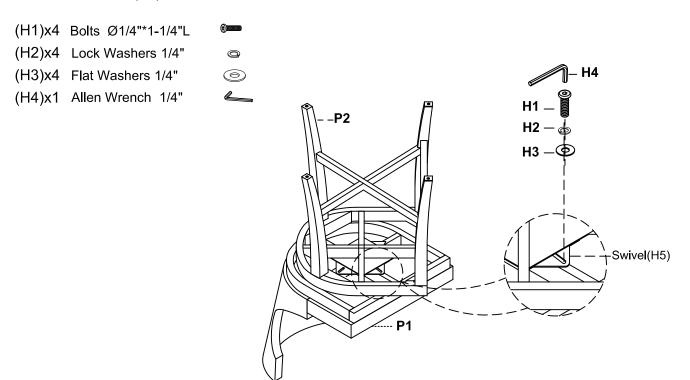
Step 2. Turn the assembled stool to an upright position. Assembly is complete. Failure to follow these instructions may cause the bolts to misalign during assembly.
