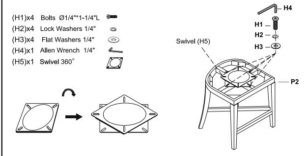
Step 2. Attach the assembled chair base (P2) to the chair top (P1) as shown below. Securely tighten all bolts with Allen wrench (H4).
