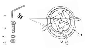
Step 4.Assemble the last leg(P2), Tighten the hardware as in the previous steps.
