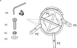
Step 3.Then using bolts(H1),lock washers (H2), flat washers (H3), connect wooden ring(P3) to legs (P2). Tighten bolts (H1) with allen wrench (H4).
