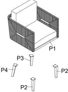
2) Attach Back leg right (P3), Back Leg left (P4) to Chair top (P1) using Allen key (H4), Lock washer (H2), Flat washer (H3), and 20 MM Bolt (H1).
