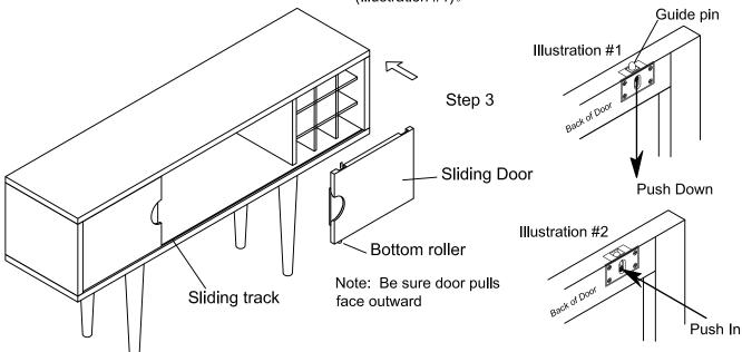
b. Place the rear door bottom rollers in the back bottom track. Pivot the top of the door to align the top guide pins with the back upper track on the console. Push the button on the back of the top guide pins to release the lock allowing the pins to pop into the top guide track. (Illustration#2) Repeat with the other door in the front set of tracks.
